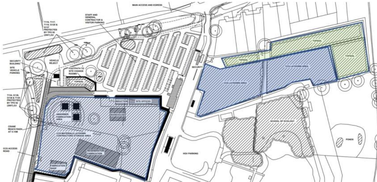
Figure 6-2. Temporary Laydown and topsoil storage areas (215000-00190-000-COS-00001)
