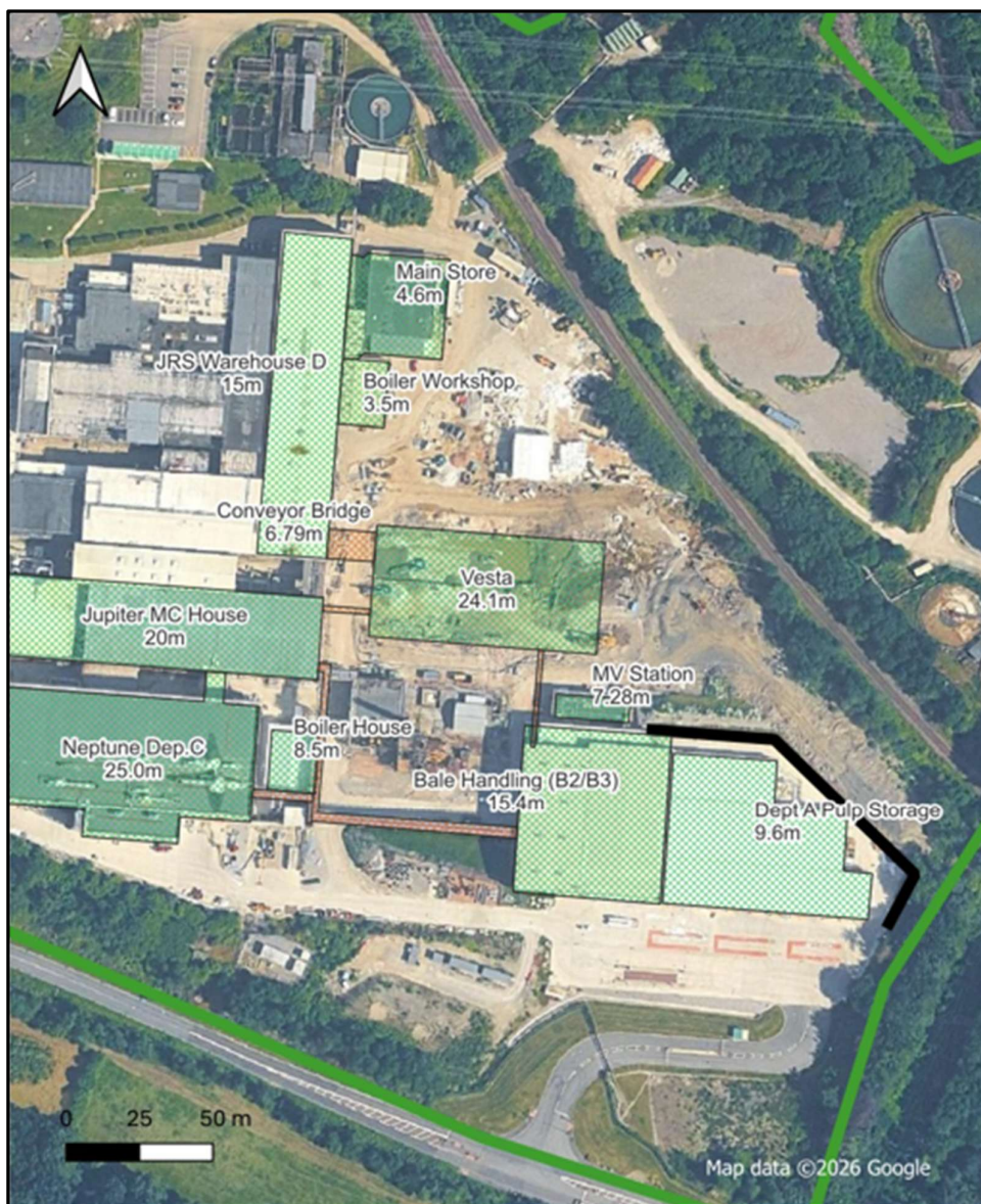
Figure 4.4 Location and Heights of Buildings that Will Affect Dispersion from the Proposed Vesta Stack
