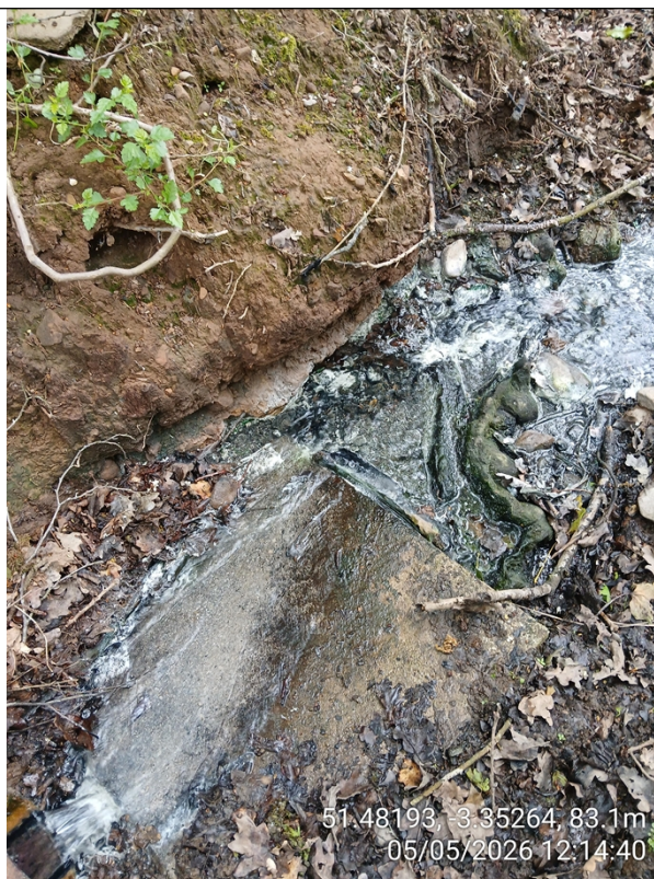
Discharge point close-up and sewage fungus
