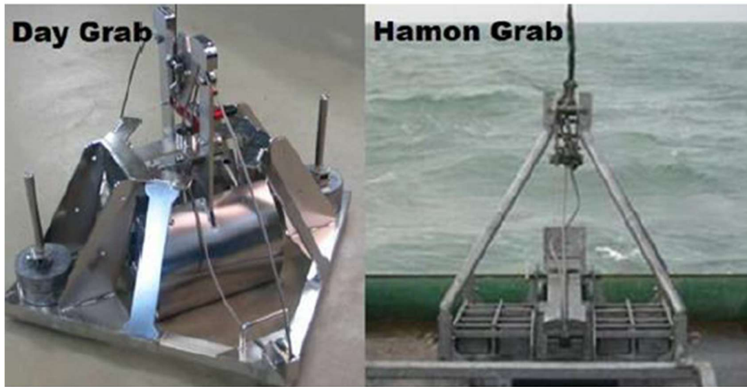
Figure 2.2: Examples of grab samplers
