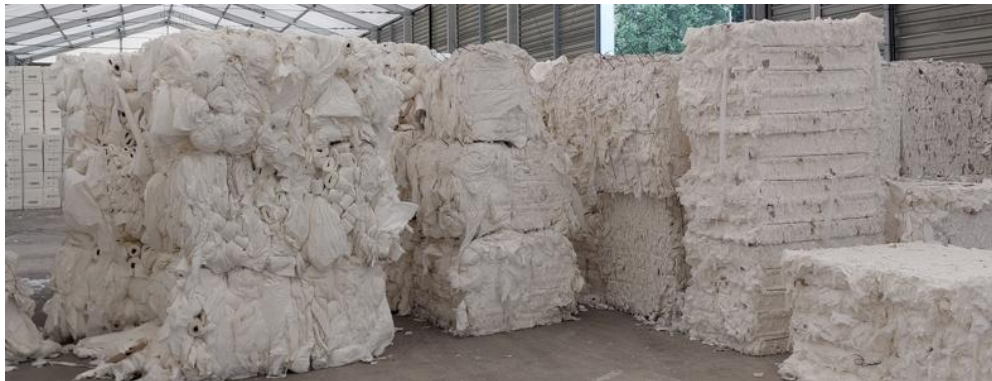
Photograph 1-3: Broke storage bales
