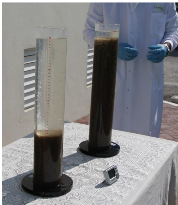
Figure 11: Demonstration of HYBACS sludge settlement at Tubli WPC
