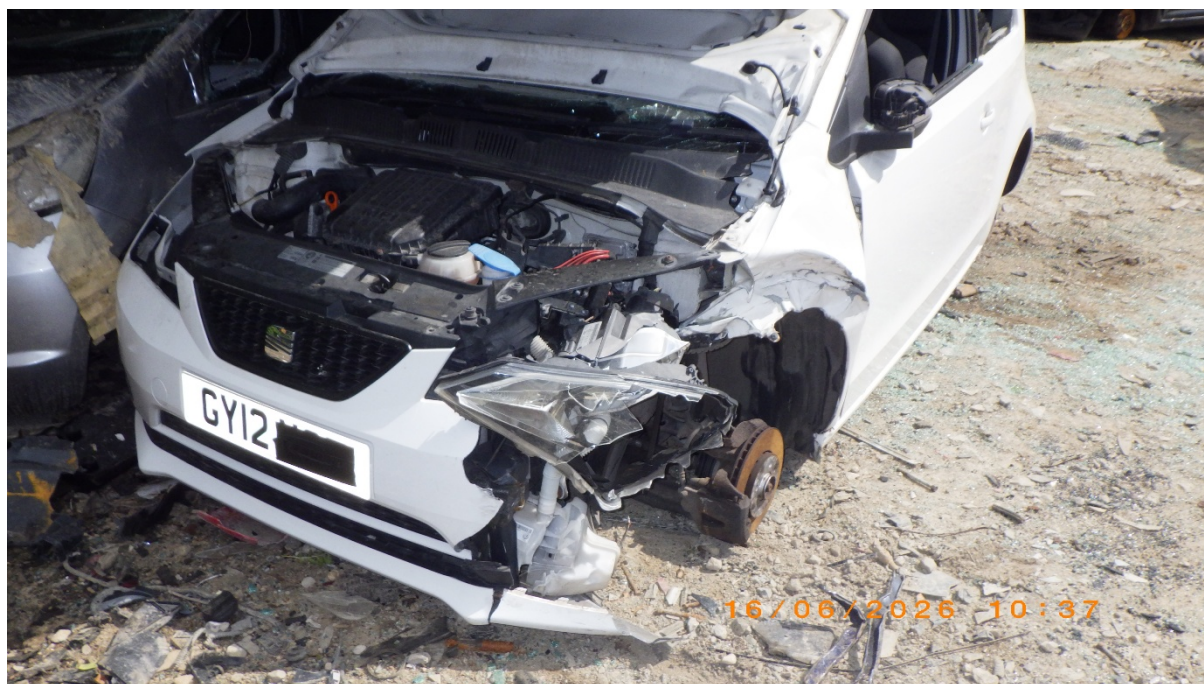
Not fully depolluted ELV stored on hardstanding surface
