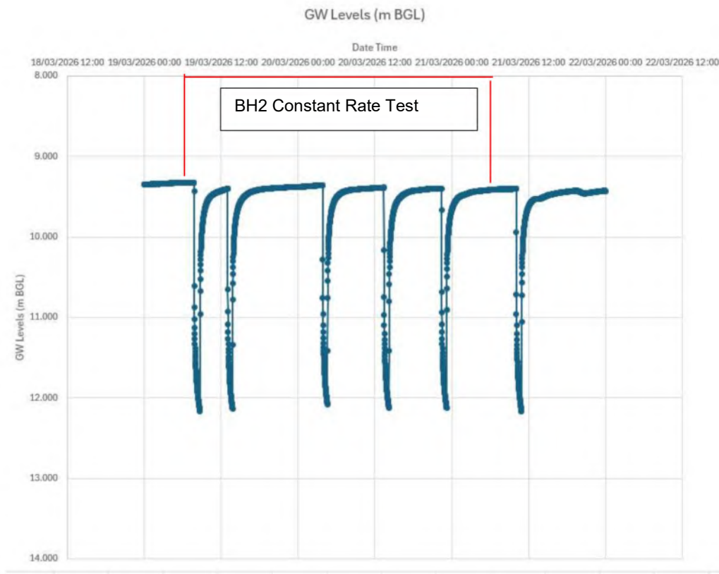
Figure 3-5 BH6 Groundwater Levels During BH2 Constant Rate Testing
