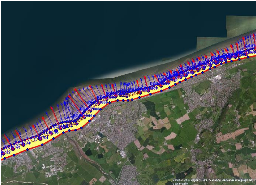
Figure 7-3: Illustration of Unibest profile density (blue lines), with comparison against measured profiles (red lines)
