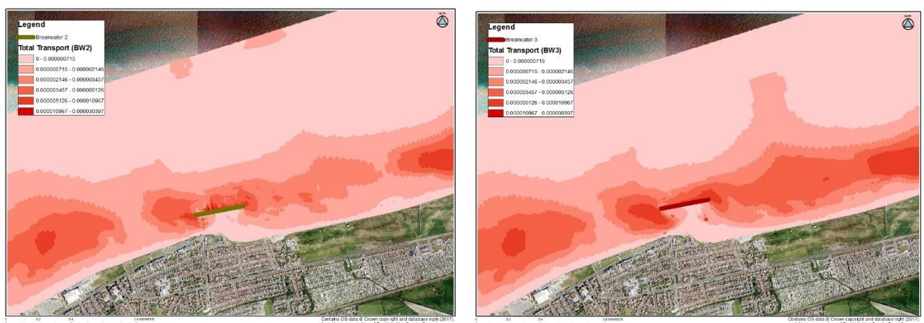
Figure 5-9: Change in mean total transport for the complete simulation between breakwater position 2 and 3 for a modelled 28-day period
