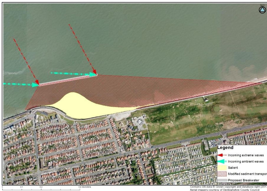
Figure 3-2: Sheltering of the shoreline under average ambient wave conditions
