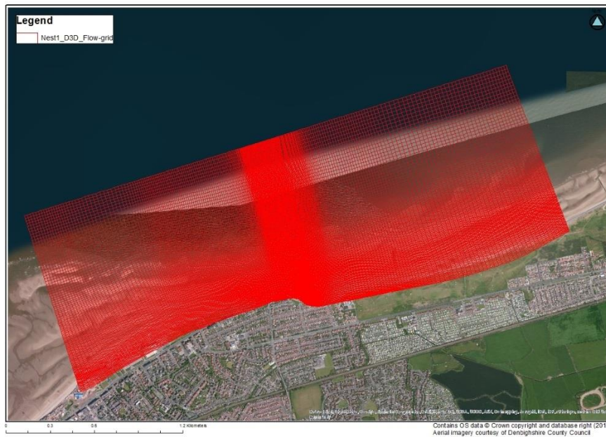
Figure 4-2: Delft3D nested model grid
