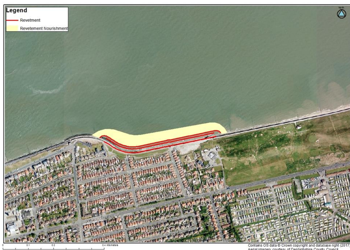
Figure 3-5: Modelled revetment and nourishment area (20,000m 2 )
