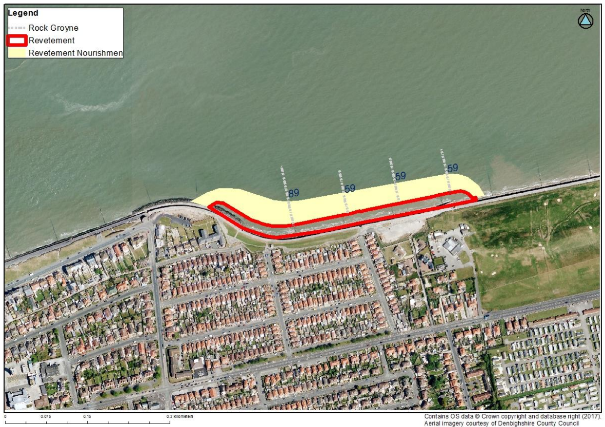
Figure 3-6: Modelled revetment and nourishment area with cross shore groynes (length denoted in meters)
