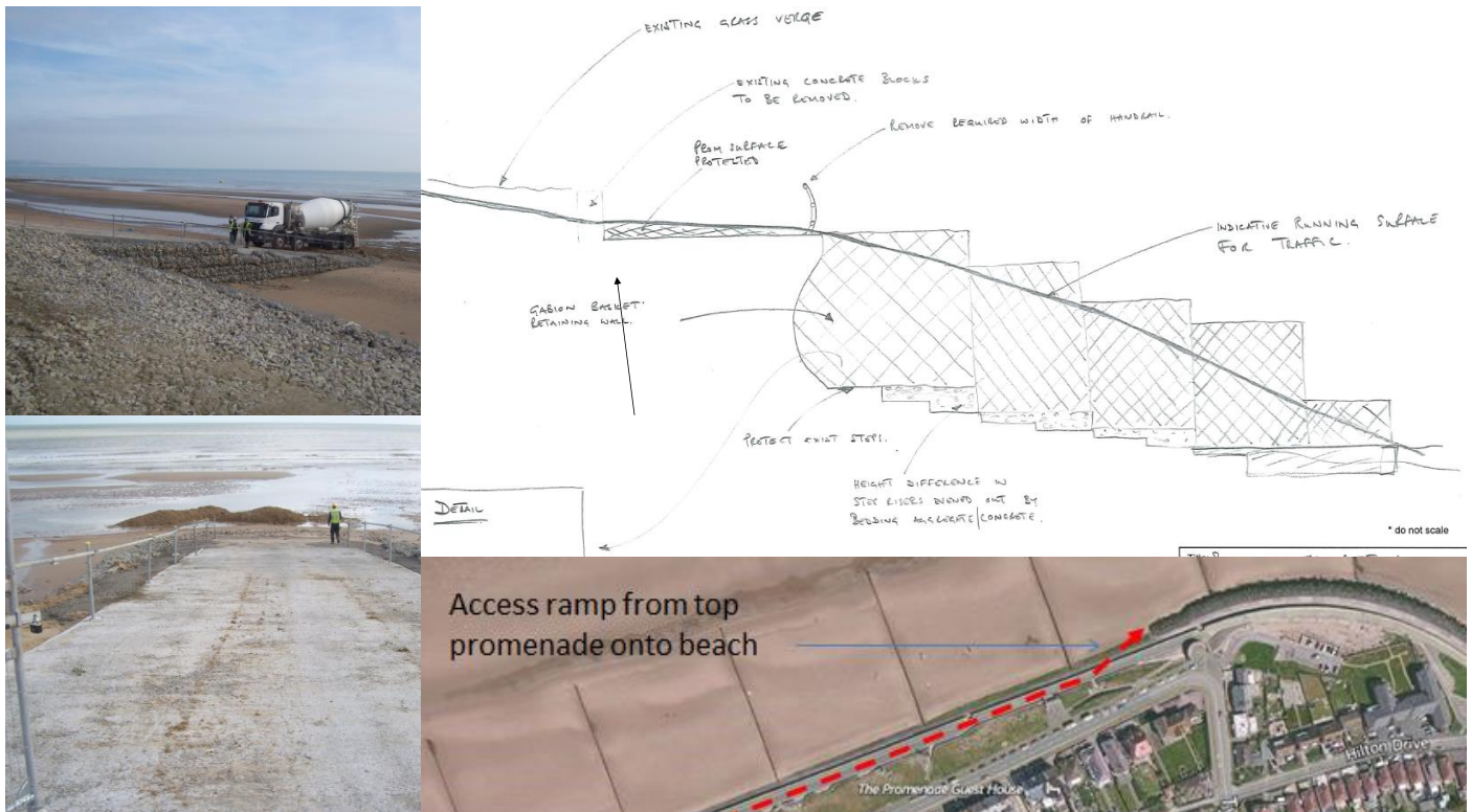
Figure 13- Temporary gabion retained slipway access near splashpoint
