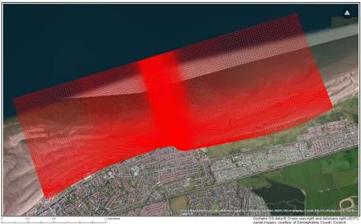
Figure 4-4: Delft3D nested model grid
