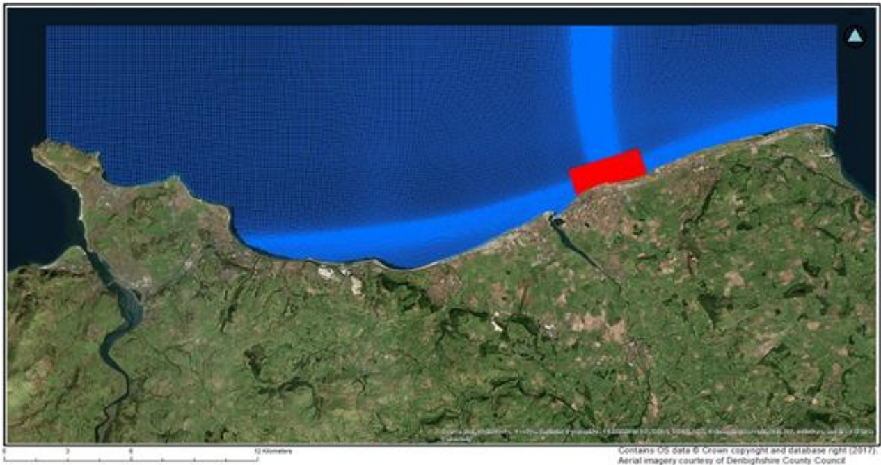
Figure 4-3: Large Delft3D model grid with nested grid (red box), from Great Ormes head (west) to Point of Ayr (east)
