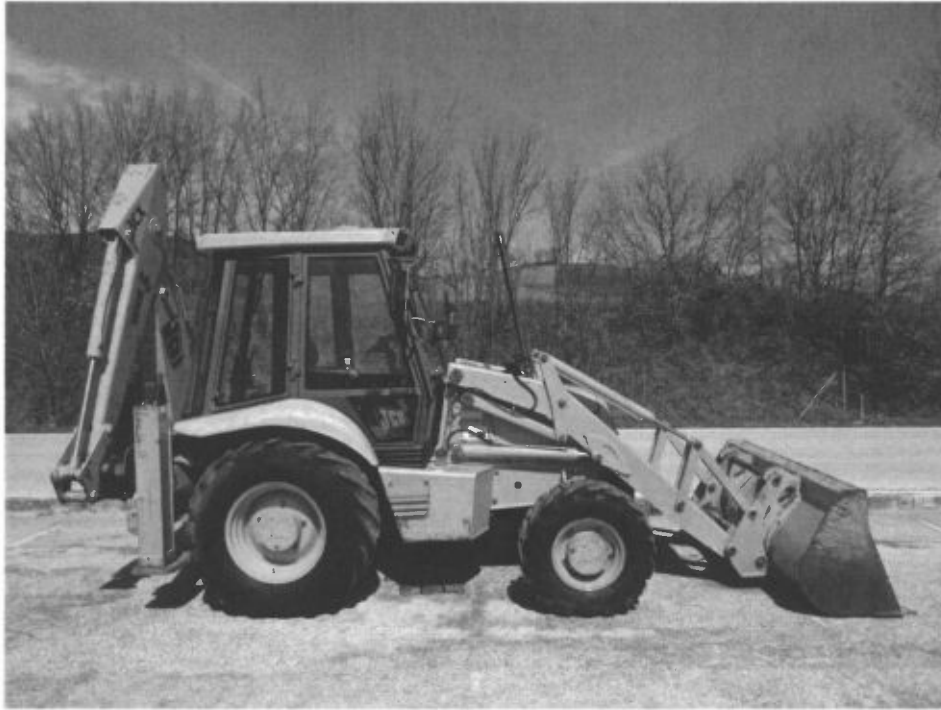
JCB with backhoe and shovel for digging trial pits.
