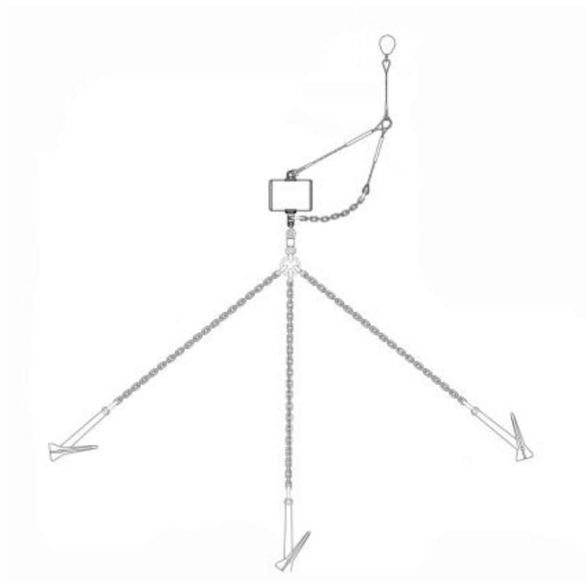
Photo 5- Typical Breasting Mooring Arrangement for All Weather Lifeboats with 3 anchors, to central mooring buoy and pick-up float (Licensable activity 1)
