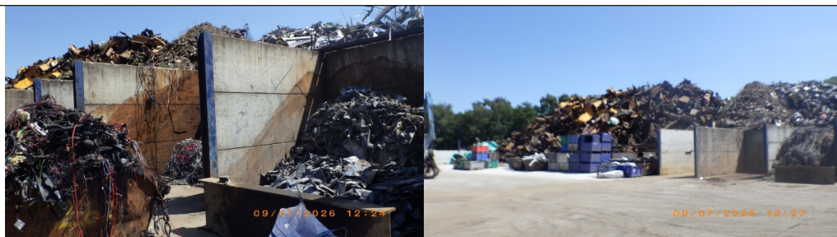
Waste piles heights significantly above the dividing wall levels
