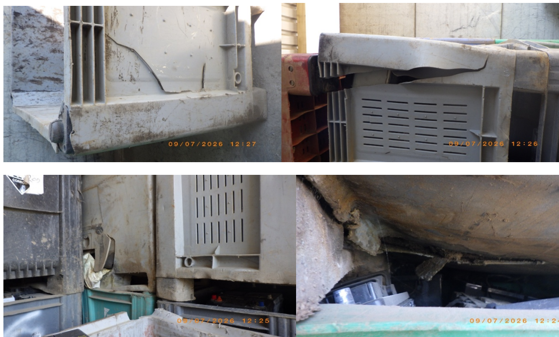
Damaged storage boxes containing waste batteries
