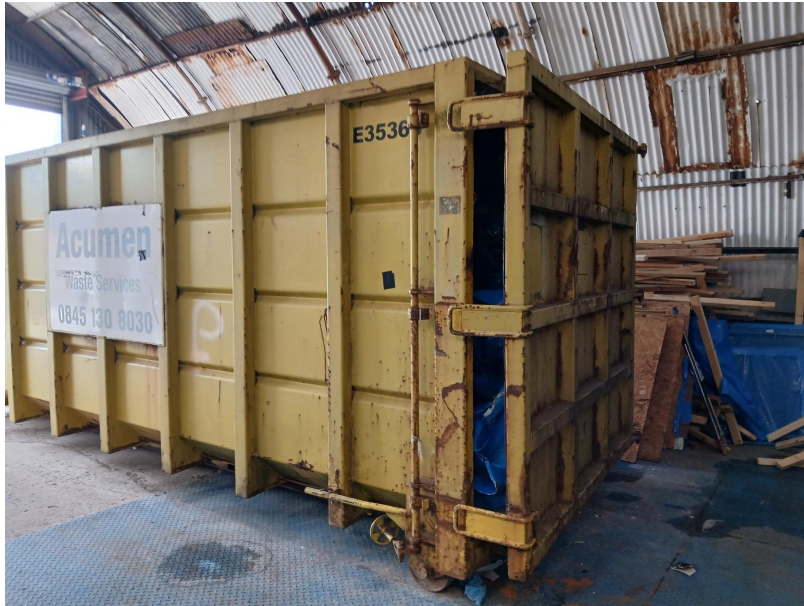
Figure 1: Unlocked asbestos waste skip
