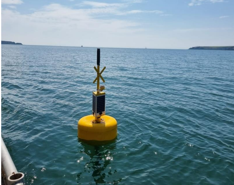
Figure 3 A data buoy like this one pictured will be moored nearby within the Warrior Way site on a single point mooring to remotely collect data from the turbines and mark the site. It will be yellow, with a St Andrews Cross and yellow flash characteristic (Fl Y 4s).
