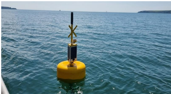
Figure 2 A data buoy like this one pictured will be moored on a single point mooring nearby within the Warrior Way site to remotely collect data from the turbines and mark the site. It will be yellow, with a St Andrews Cross and Yellow Flash Characteristic (Fl Y 4s)
