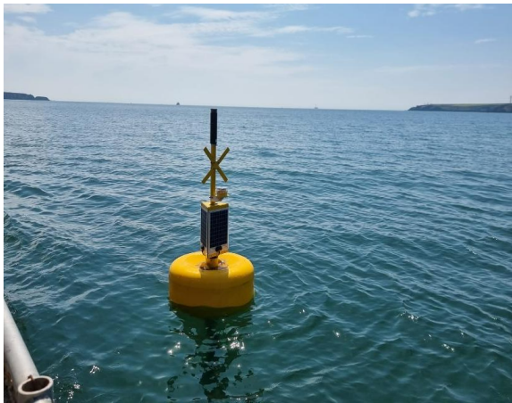
Figure 3 A data buoy like this one pictured will be moored nearby within the Warrior Way site on a single point mooring to remotely collect data from the turbines and mark the site.
