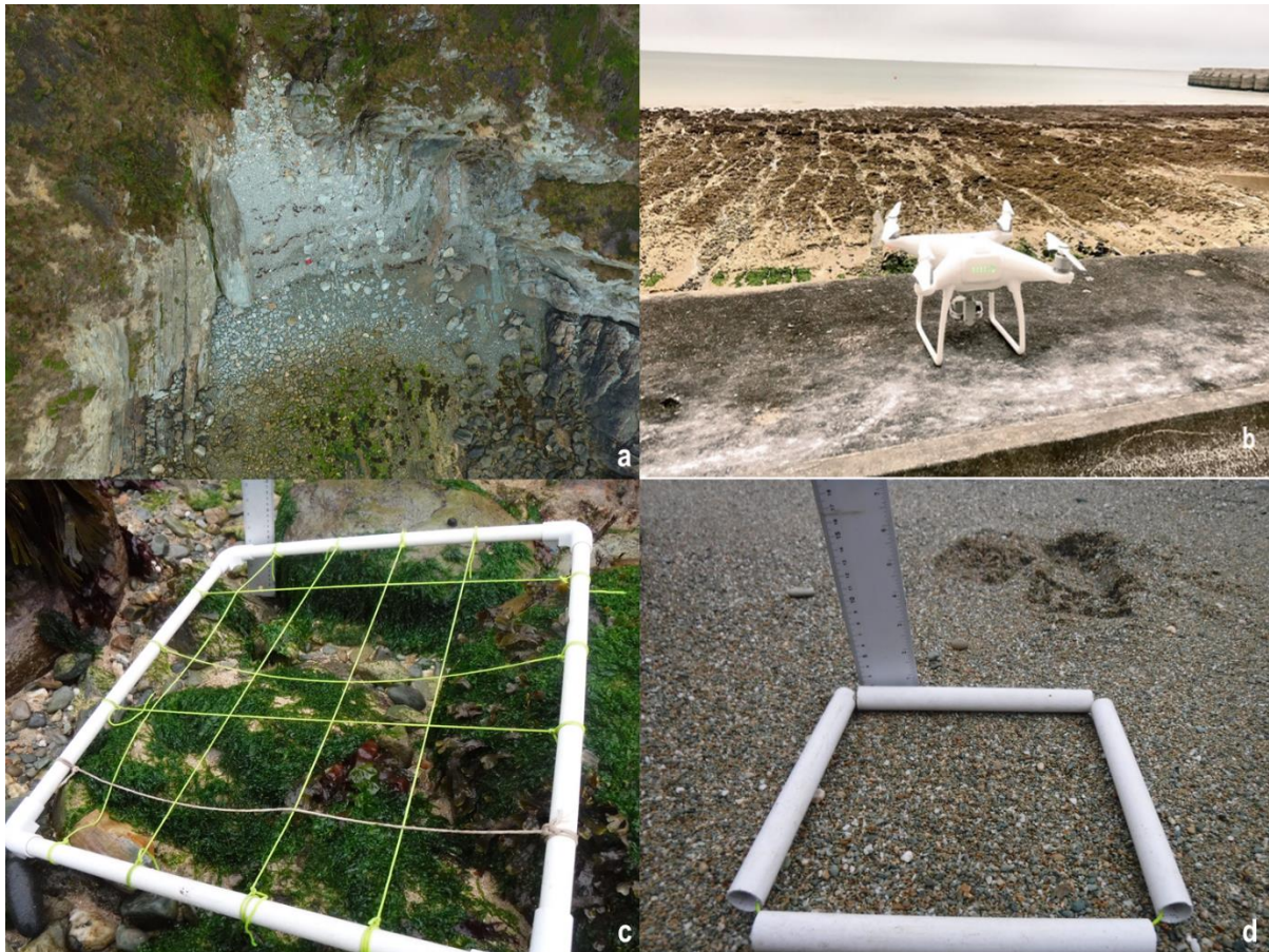
Plate 2 Intertidal sampling techniques employed during the benthic ecology characterisation survey in September 2018. a) High resolution aerial image of the upper shore. b) DJI Phantom 4 UAV used to undertake aerial mapping. c) 0.25 m 2 quadrat used to sample hard substrates. d) 0.04 m 2 quadrat used to sample soft sediments.
