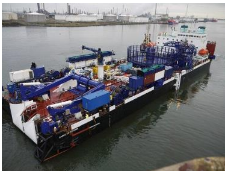
Figure 22: Cable Enterprise, cable lay barge (Image Source 4COffshore)
