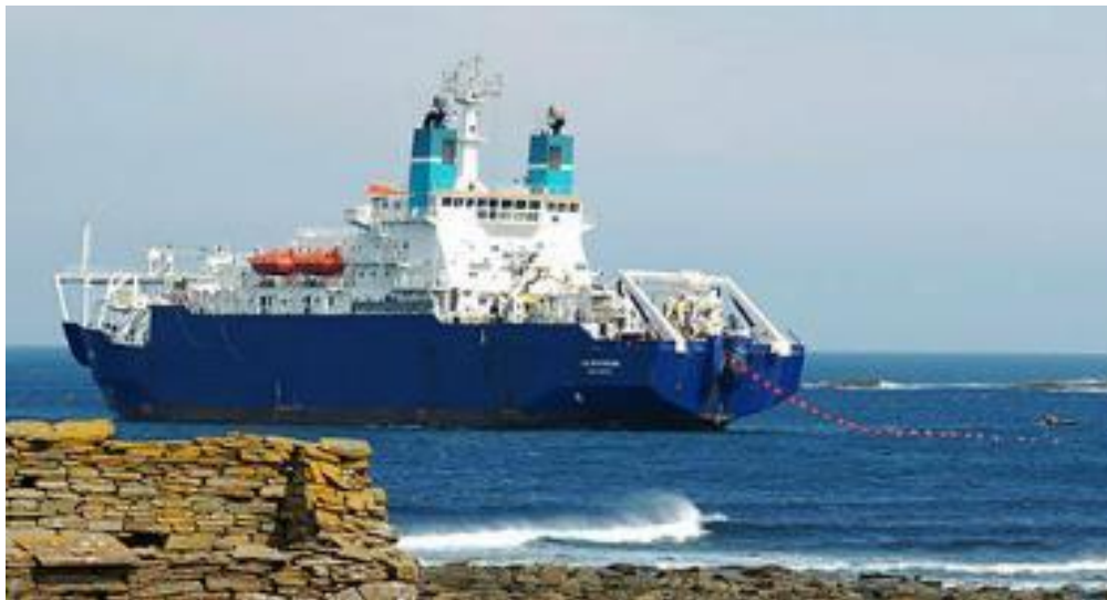
Figure 21: DP2 cable lay vessel (CLV) - C.S Sovereign (Image Source: Global Marine)
