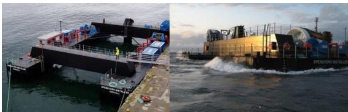
Figure 31: Open Hydro bespoke installation vesse (Image Source: Open Hydro)
