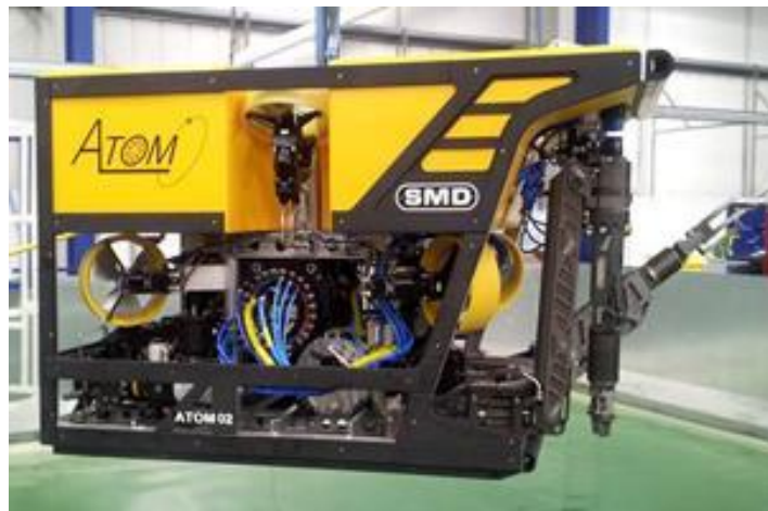
Figure 32: Work Class ROV (Image Source: SMD)
