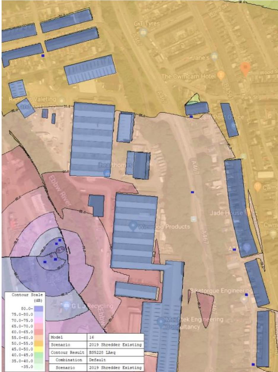
**5217/NM2 – Daytime Noise Map of Proposed Shredder/Screening Plant and Enclosure**
