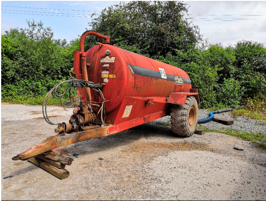
Photo 6 – 3000L Water bowser used for dust suppression in Forest Wood quarry. Currently situated near the settlement lagoon (A2) and is typically used twice a day during drier months. (26/06/19 13:37)
