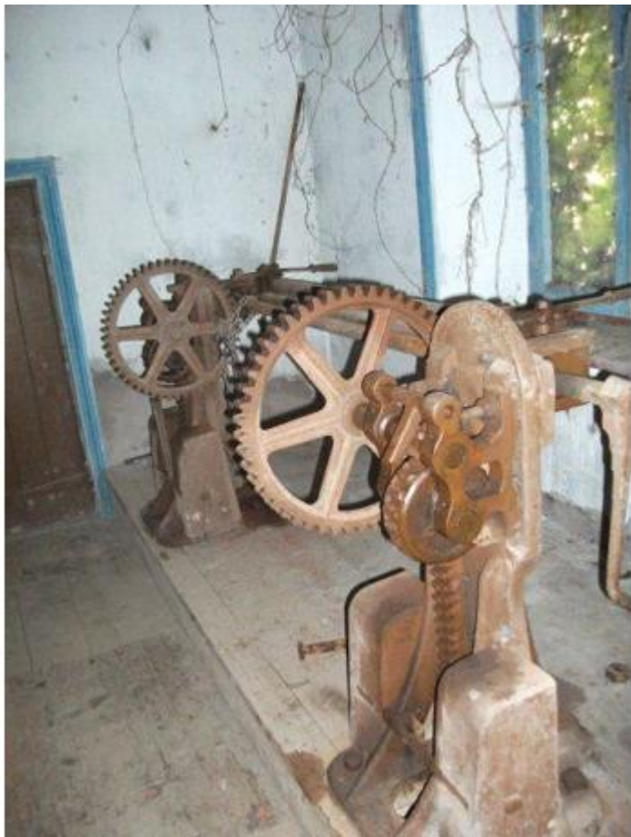
Photo 2: Sluice controls inside valve house 07.11.13
