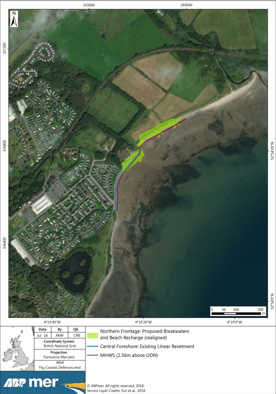
Figure 2. Outline of proposed coastal defences showing their extent relative to the position of the existing Mean High Water Spring elevation
