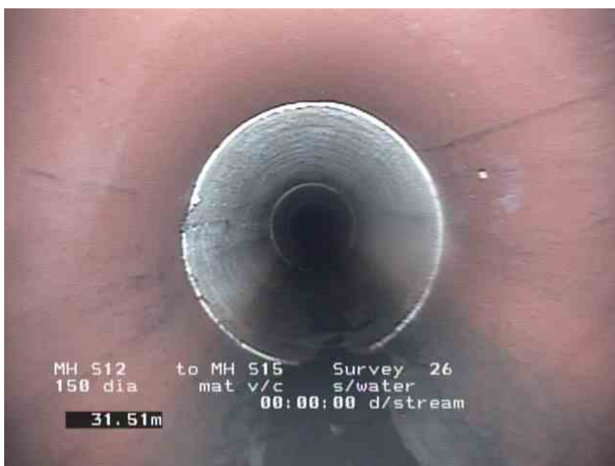
S12X_6b652c16-f3ac-4c81-866a-854d12ce5751_20190831_155341_367.jpg, , 31.87m Point repair, localised lining from 12 o'clock to 11 o'clock
