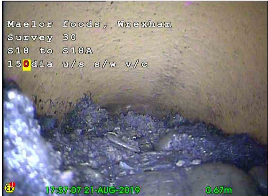
S18AX_10c15f4b-8ad3-4905-8990-d8c740d23703_20190901_143129_919.jpg, , 1.25m Settled deposits, coarse, 80% cross-sectional area loss
