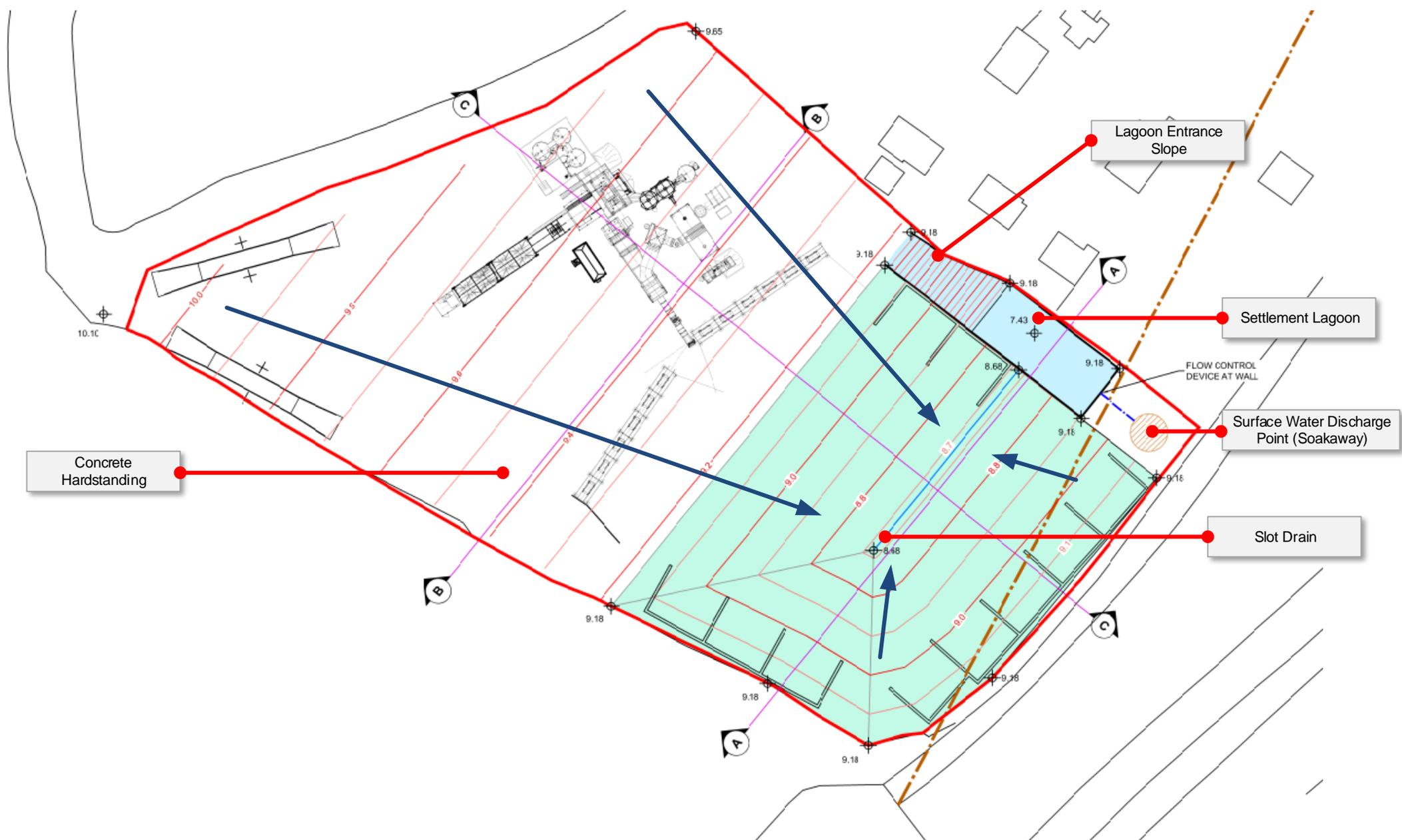
Based on Harsco (2019). SLR Surface Water Drainage, Scale 1:500 @ A2, DWG No. 001, DRAFT, Revision D0, June 2019
