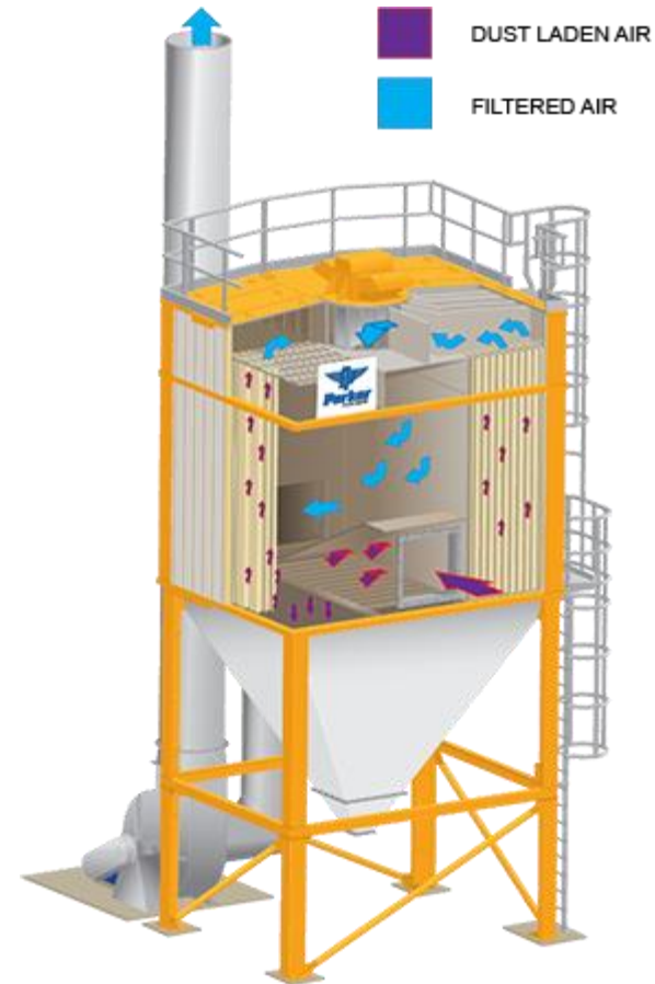
Figure 4: Secondary dust collection system (bag filter)
