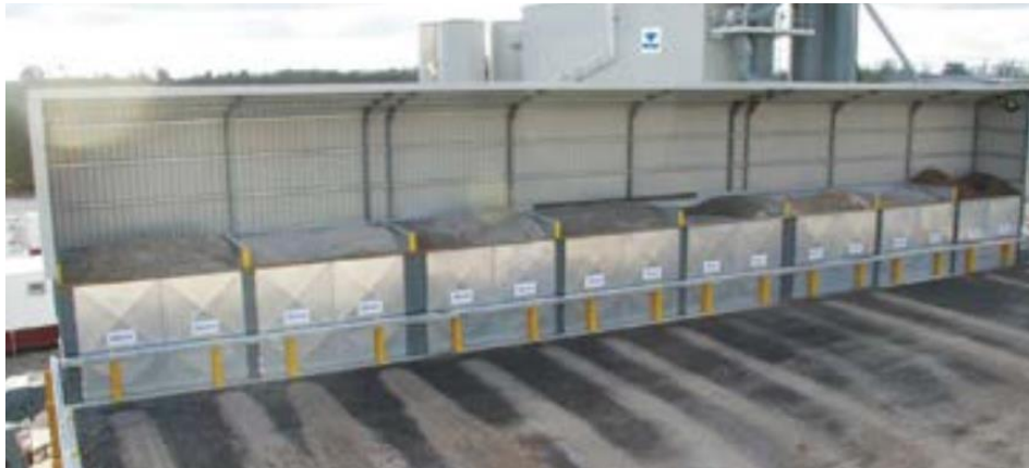
Photograph 4-2: Typical aggregate cold feed unit
