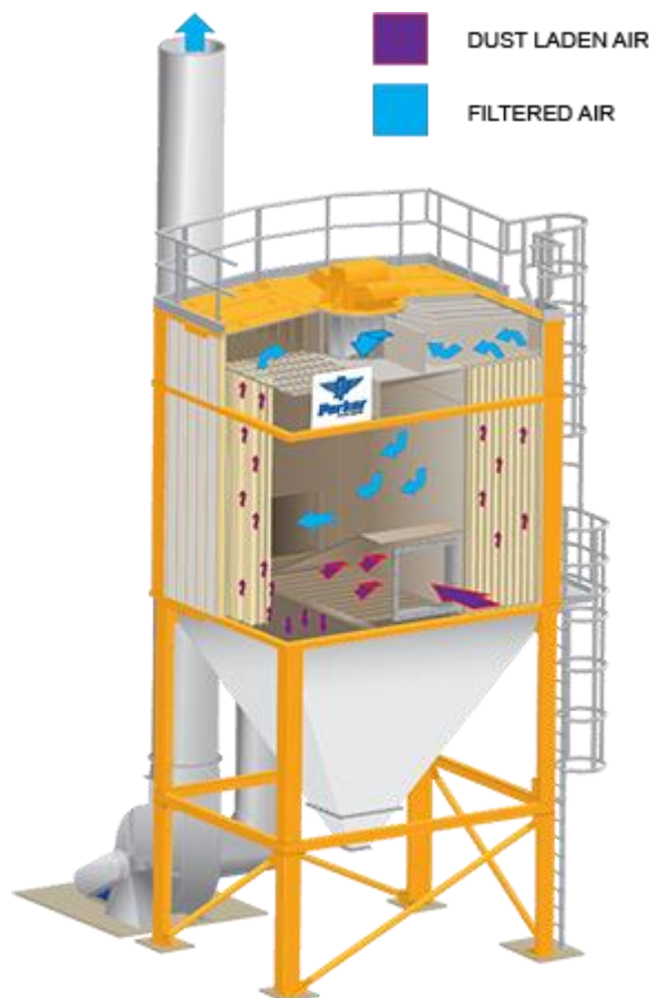
Figure 4-4: Secondary dust collection system (bag filter)
