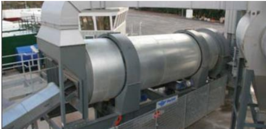
Photograph 4-3: Typical aggregate dryer
