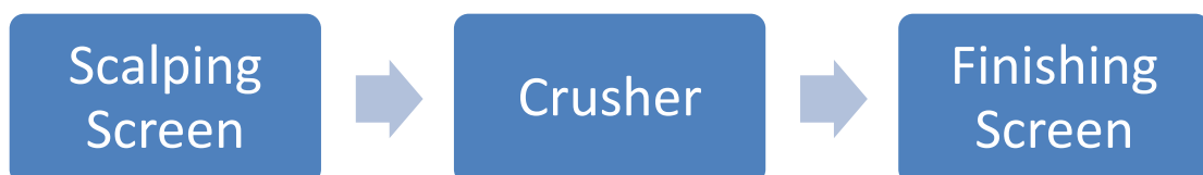
Figure 3-1: Slag screening and crushing process
