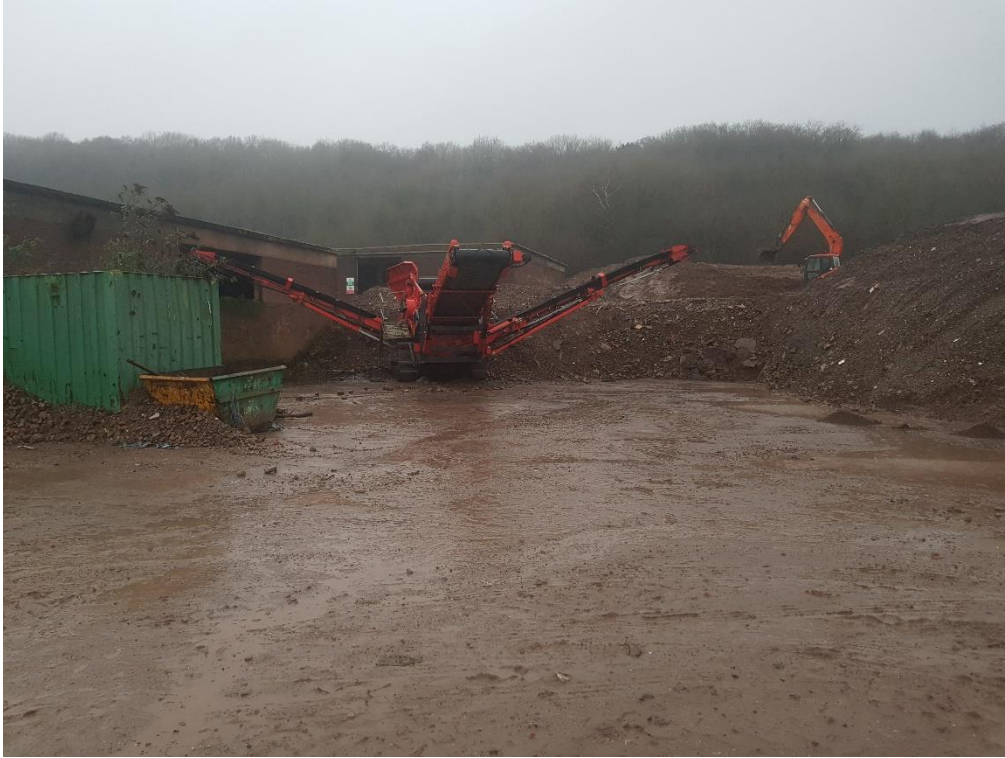
Screen on hardstanding at the eastern end of Building 5 – screened topsoil is loaded into the building through the hole on the eastern wall of the building.
