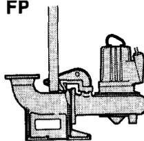
For permanent installation, a system with guide bar and discharge connection fixed to the sump floor or pump well is used. When the pump is lowered down the guide bars it engages automatically with the discharge connection — and automatically released when it is raised.
