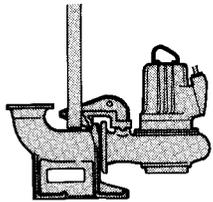
This system with guide bar and discharge connection permits automatic connection of the pump to the discharge line. The unit can be removed for inspection without anyone having to enter the sump.
