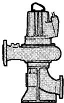
The pump is installed dry on a base stand and is connected directly to the inlet and outlet lines. The submersible design of the pump prevents damage in the event of flooding.
