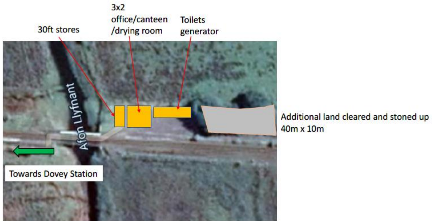
Typical site layout at Dovey Junction Station
