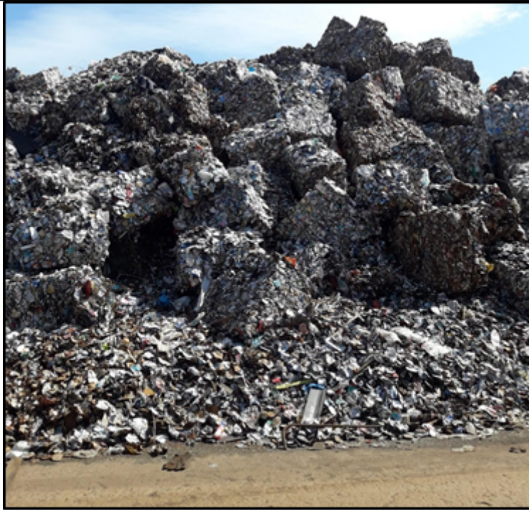
Image 4 – showing baled metal material stored in piles in excess of 4 metres in height
