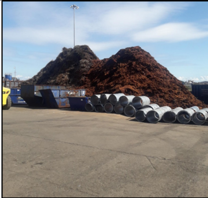
Image 2 – showing non-combustible material stored in excess of 4 metres in height
