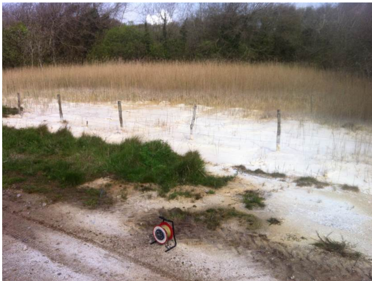
Plate 6-3 Accumulation of secondary precipitates adjacent to MCL (between BH17 and P12)
