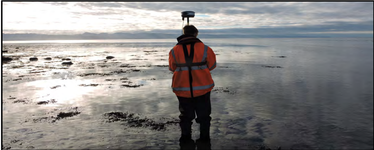
Image 3. ABPmer Ecologist using the Hemisphere S320 Global Navigation Satellite System
