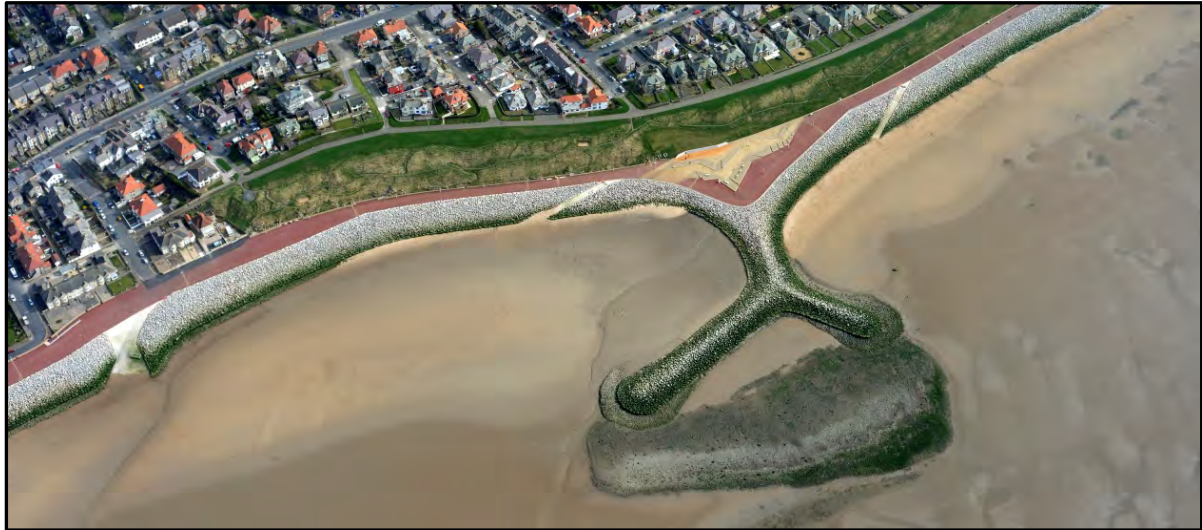
Image 19. Breakwater at Morecambe with innovative rocky habitat mitigation area in front
