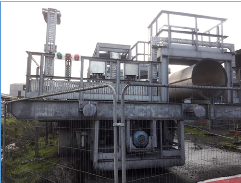
MCO's new Minister Stein fume arrestment hood ready for installation
