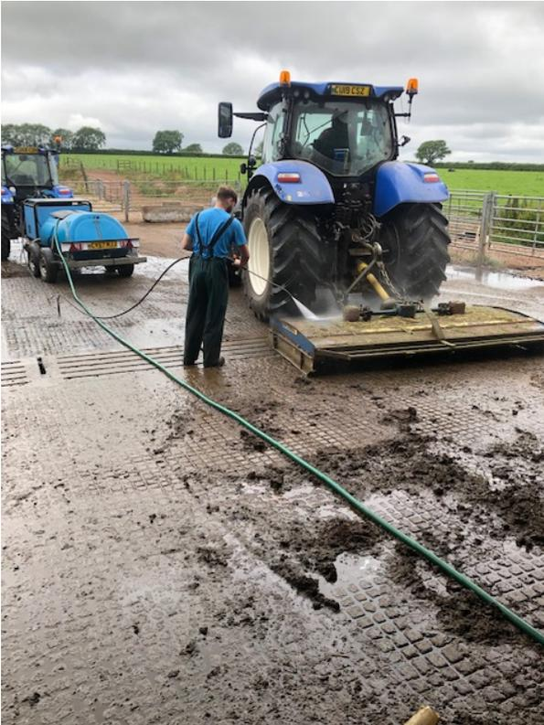
On average eight agricultural vehicles are washed down per week (maximum 2 per day) using a mobile 4,000psi pressure washer (Hyundai HYW4000P) throughout the year. Flow rate and normal wash duration (1 hour per vehicle) have been used to estimate use.
