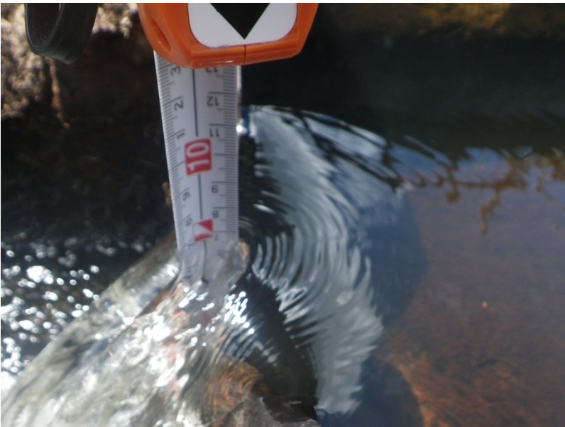
Measurement of compensation flow over v-notch
