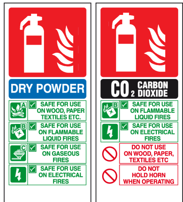
Figure 2: Fire Extinguishers Type and Application
