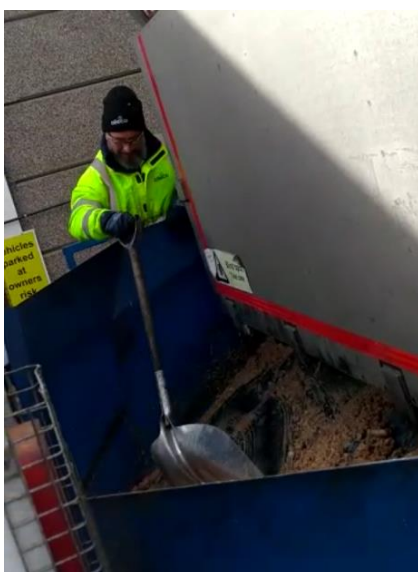
Fig 4a shows an operator using his shovel to scrape residual food waste down the chute into the compactor
