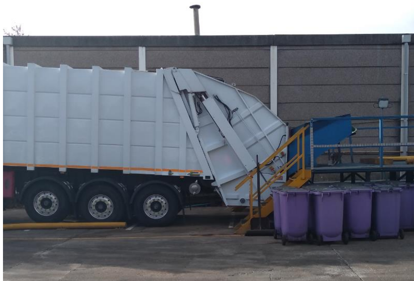
Fig 3a shows the Goliath trailer in the correct position beneath the food waste chute
