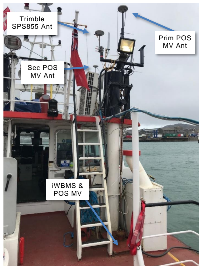
Figure 3 Position of GNSS antennas and iWBMS
