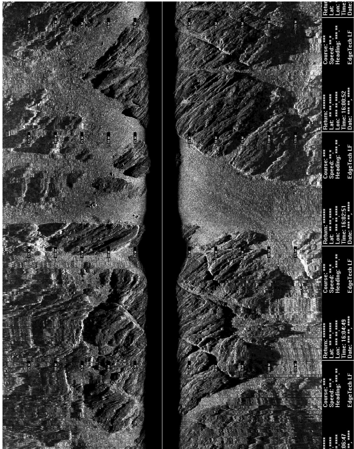
Figure 17 Low frequency (100kHz) side scan sonar data example
