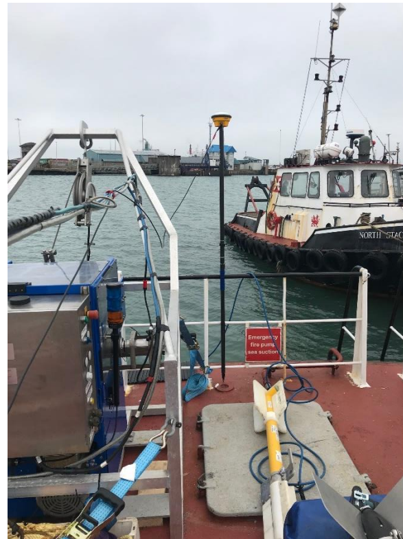
Secondary Trimble antenna on the stern
