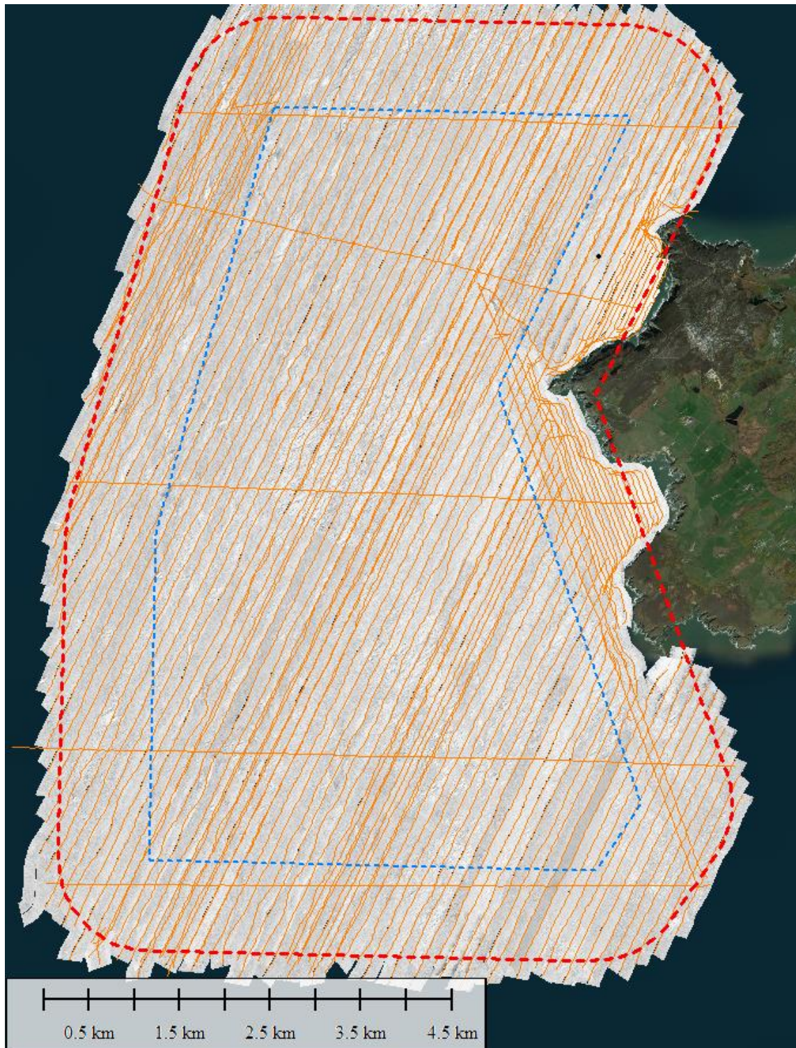
Figure 13 Side Scan Sonar Coverage and Track Plot
