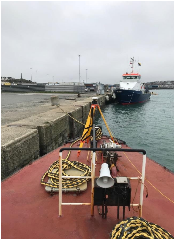
Primary Trimble antenna on the bow
