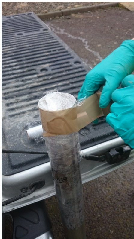
Figure 2 - Cores selected for freezing were sealed at the base using a plastic cap before further sealing with plastic film and tape to prevent water loss
