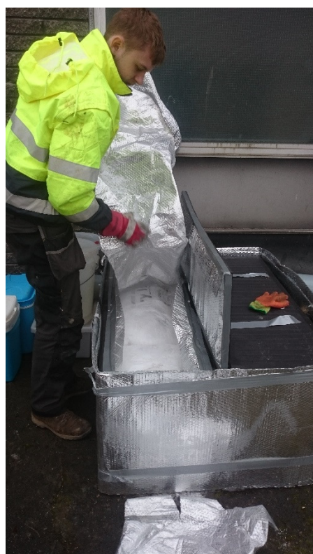
Figure 4- Insulated caskets prepared for the storage of dry ice were also used to store frozen cores.
