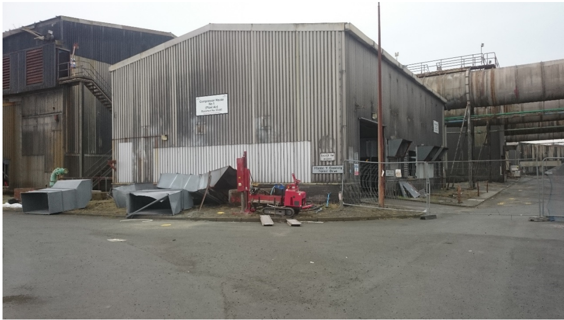
Figure 1 - Compressor house building and area of frozen core collection. Percussive drilling rig used to obtain core samples is visible in the midground here.
