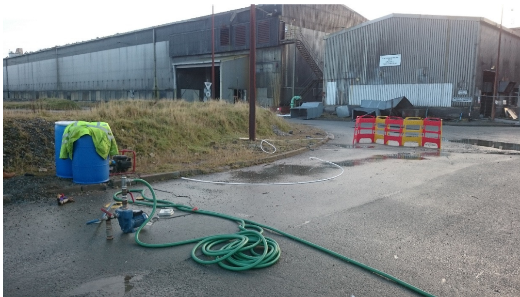
Figure 7 - Hydraulic testing was undertaken on selected boreholes to determine aquifer properties. Here, a step test is in progress in the Compressor House area drawing from RBH528a. Pressure transducers have been placed in the extraction well and in wells in the surrounding area to monitor changes in hydraulic head.
