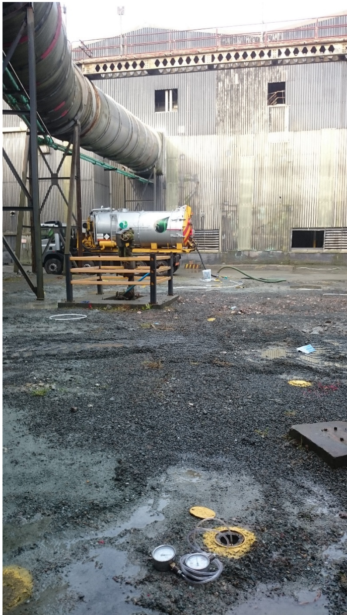
Figure 9 - Vacuum testing being carried out in the Compressor House area using a vacuum tanker. Here, RBH514a is being drawn from at 4bar. Changes in pressure in surrounding wells are being monitored using pressure gauges visible in the foreground of the above photograph.
