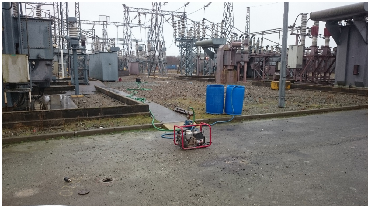
Figure 8 – Once identified and investigated, hydraulic testing was undertaken on selected boreholes to determine aquifer properties. Here, a falling head test is in progress in the Rectifier Yard. Pressure transducers have been placed in the injection well and in wells in the surrounding area to monitor changes in hydraulic head.
