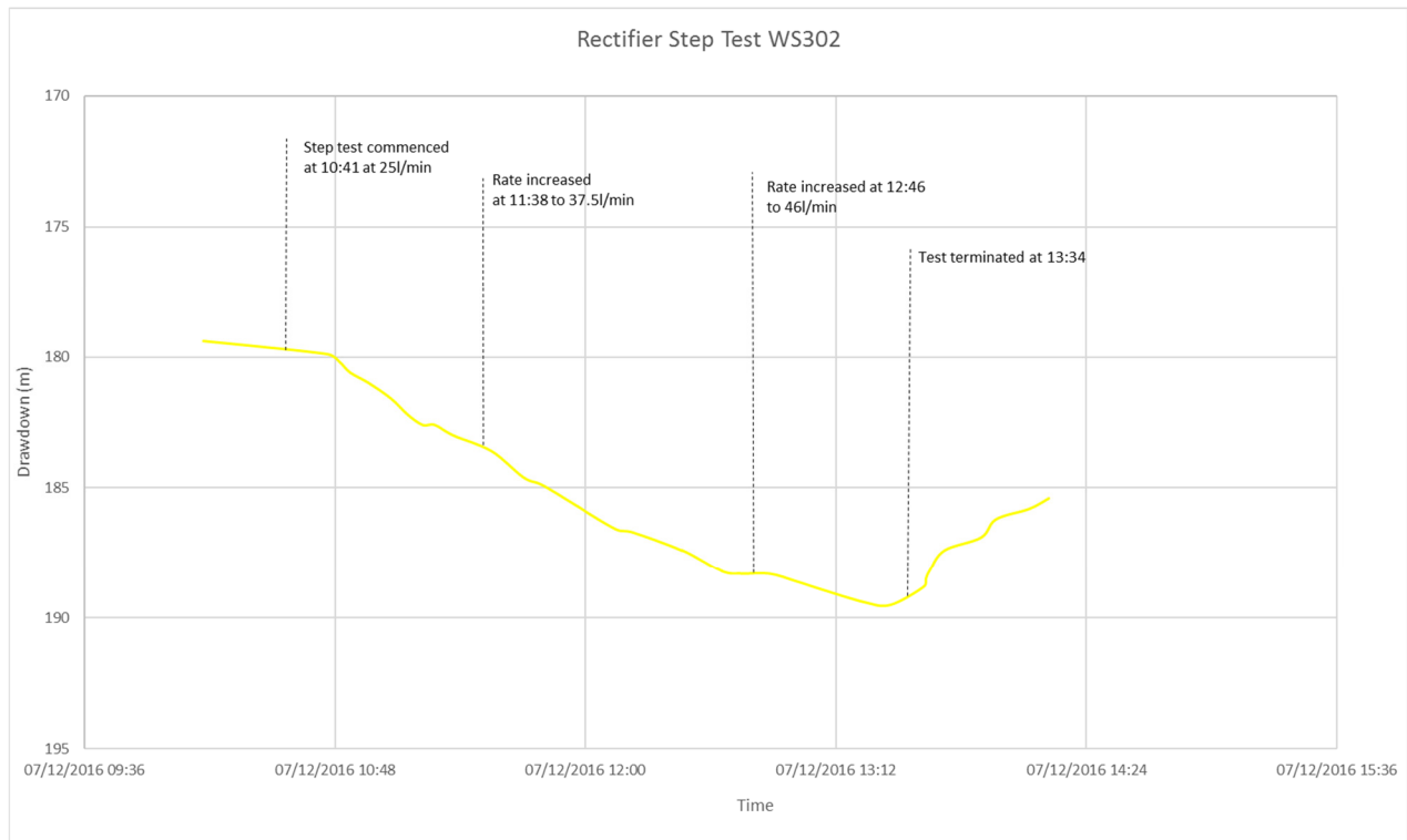
Graph 6 - Graph detailing changes in hydraulic head in WS302 during the step test conducted in the Rectifier Yard area. The drawdown axis has been adjusted from that used in Graph 12 to better graphically illustrate the impact of pumping from WS301 on WS302
