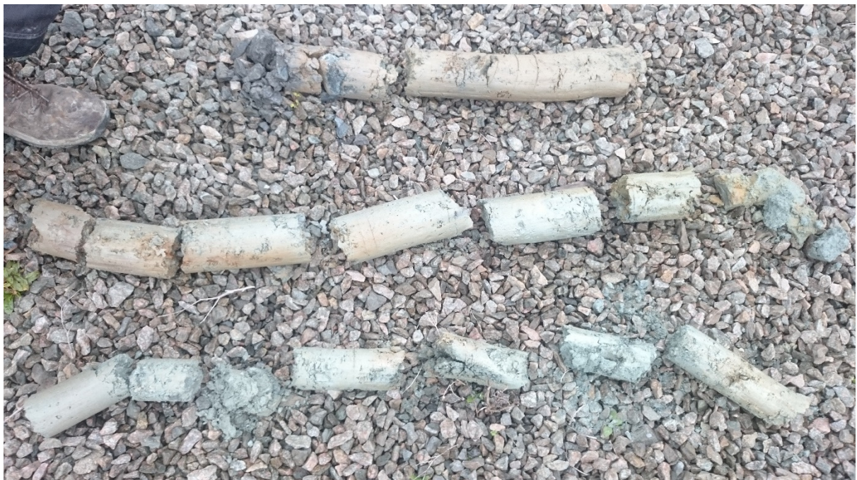
Figure 2 - Example of subsoils extracted during drilling works in the Rectifier Yard area. Blue, silty weathered schist can be seen in the lower third of the photograph. These cores had been removed from plastic sleeves. Cores to be frozen were left intact.
