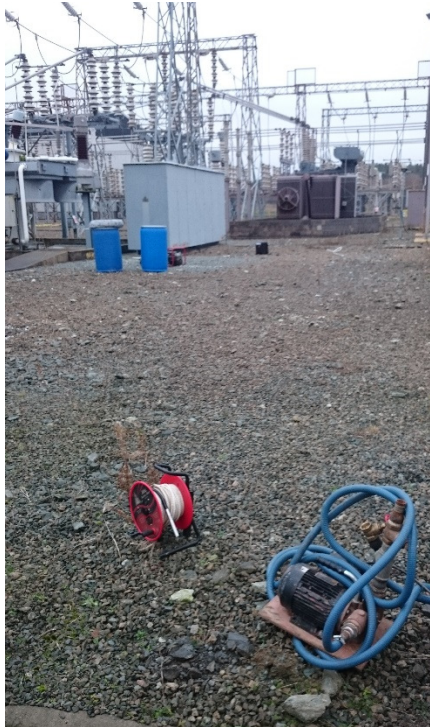
Figure 7 - Ideal locations for hydraulic testing were identified prior to arrival onsite, monitoring using an interface probe was undertaken during the works to confirm these locations or to select alternative areas for study. The wells in the above photograph were located in the Rectifier Yard area.
