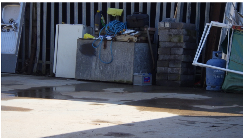
Battery on site not in sealed/covered container.
