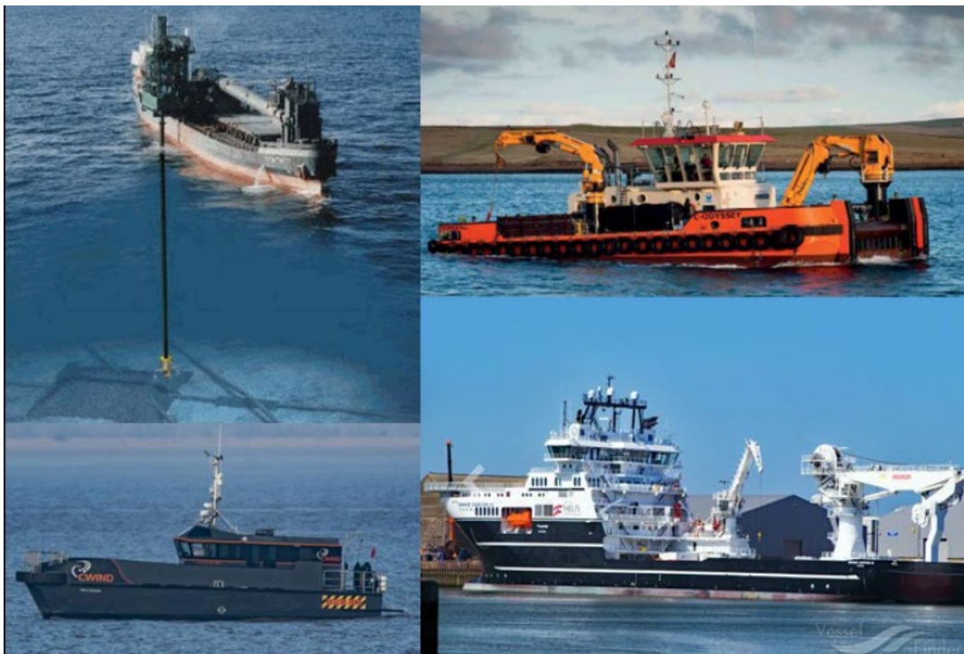
Clockwise from left: Fall pipe vessel, construction support vessel, dive support vessel, crew transfer vessel
