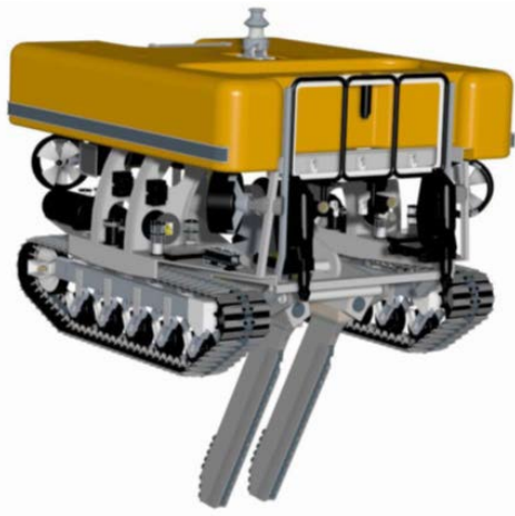
Figure 2-3 Typical water jetting machines
