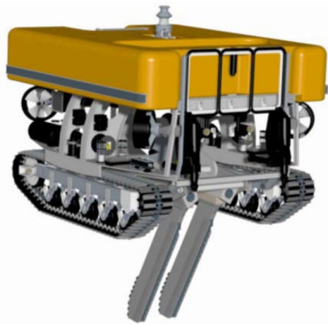
Figure 2-3 Typical water jetting machines
