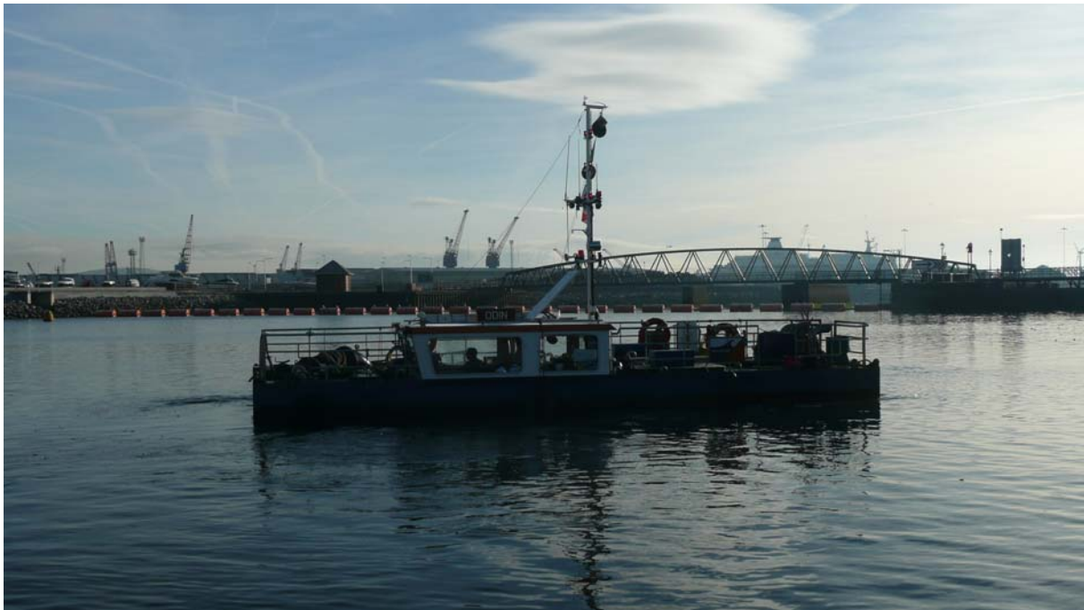
Figure 5: Self-propelled water injection dredger working in SYCAC Marina
