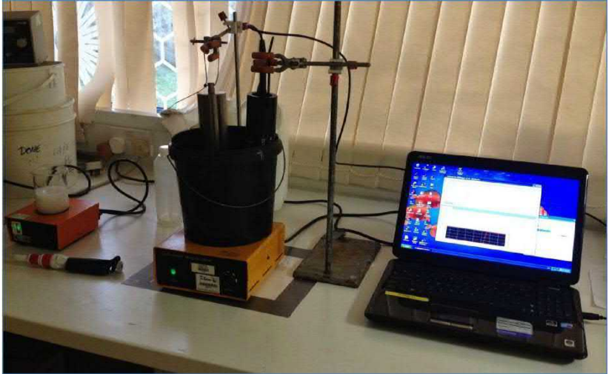
Figure 3.1 Aquatec and JFE turbidity loggers setup for adding standard additions
