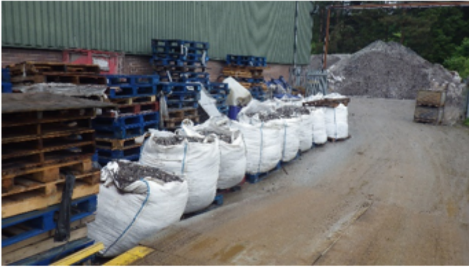
Waste 'sweepings' containing contaminated glass stored outside contrary to permit conditions
