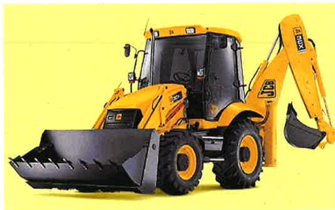
Figure 4 - JCB 3CX back-actuated excavator and shovel
