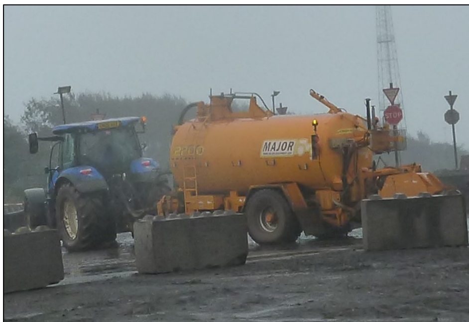
Figure 4: New dust suppression tanker with enhanced capability
